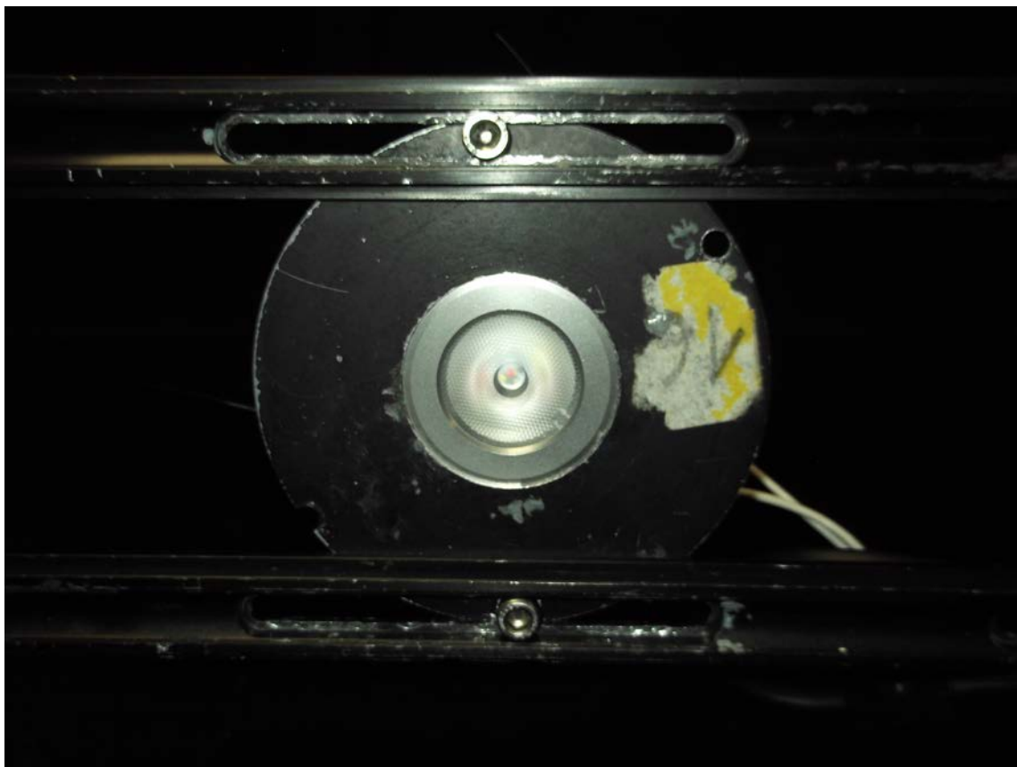
Photo 1: Luminaire on goniometer mount
